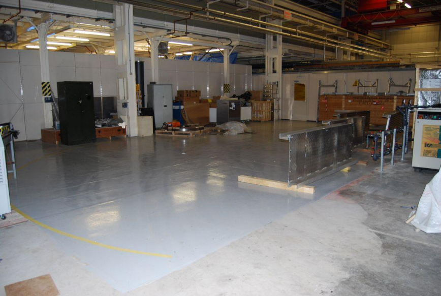
Area cleared and Yellow line for 5 Gauss limit..
