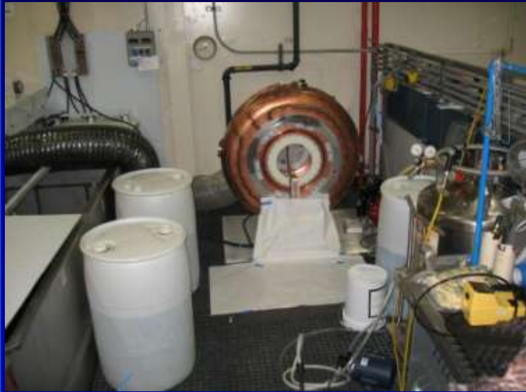
EP setup in plating shop at LBNL
