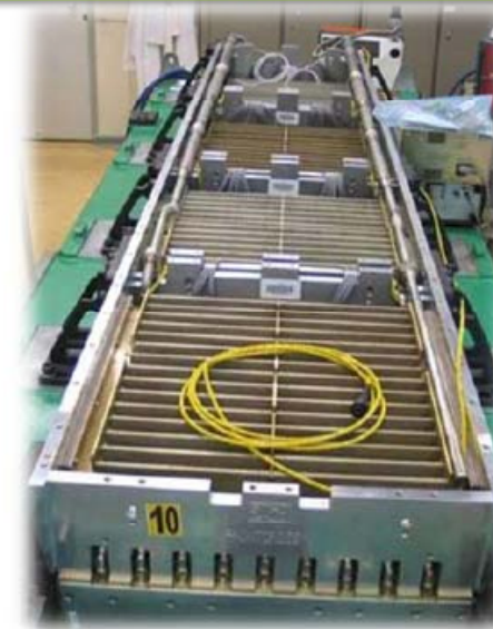
Cooling circuits installed
