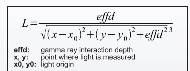
Using the appropriate variables for our currently used crystal and photomultiplier, and integrating along the different anode surfaces we get the following light distribution for each anode when an incidence happens:
