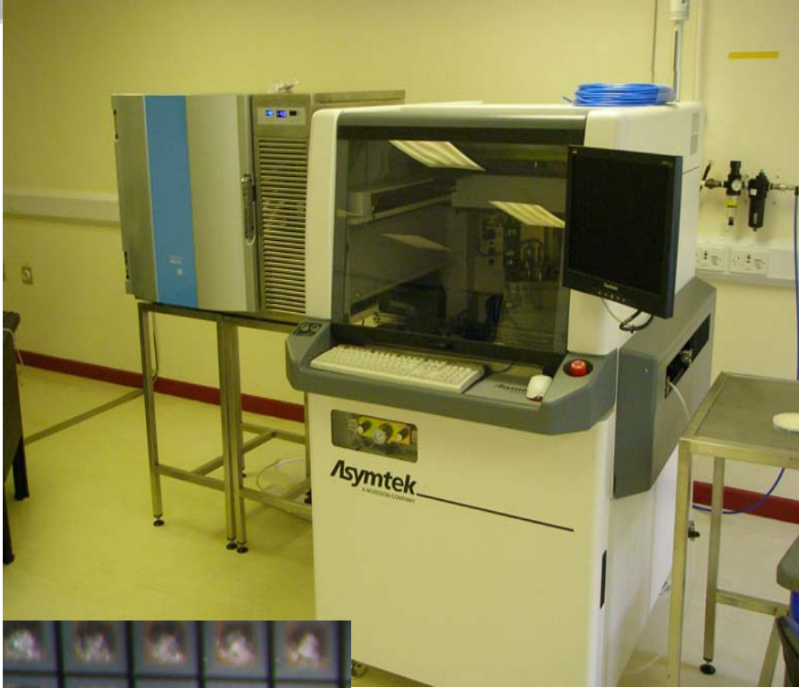
Silver loaded epoxy dispense 120um dots
