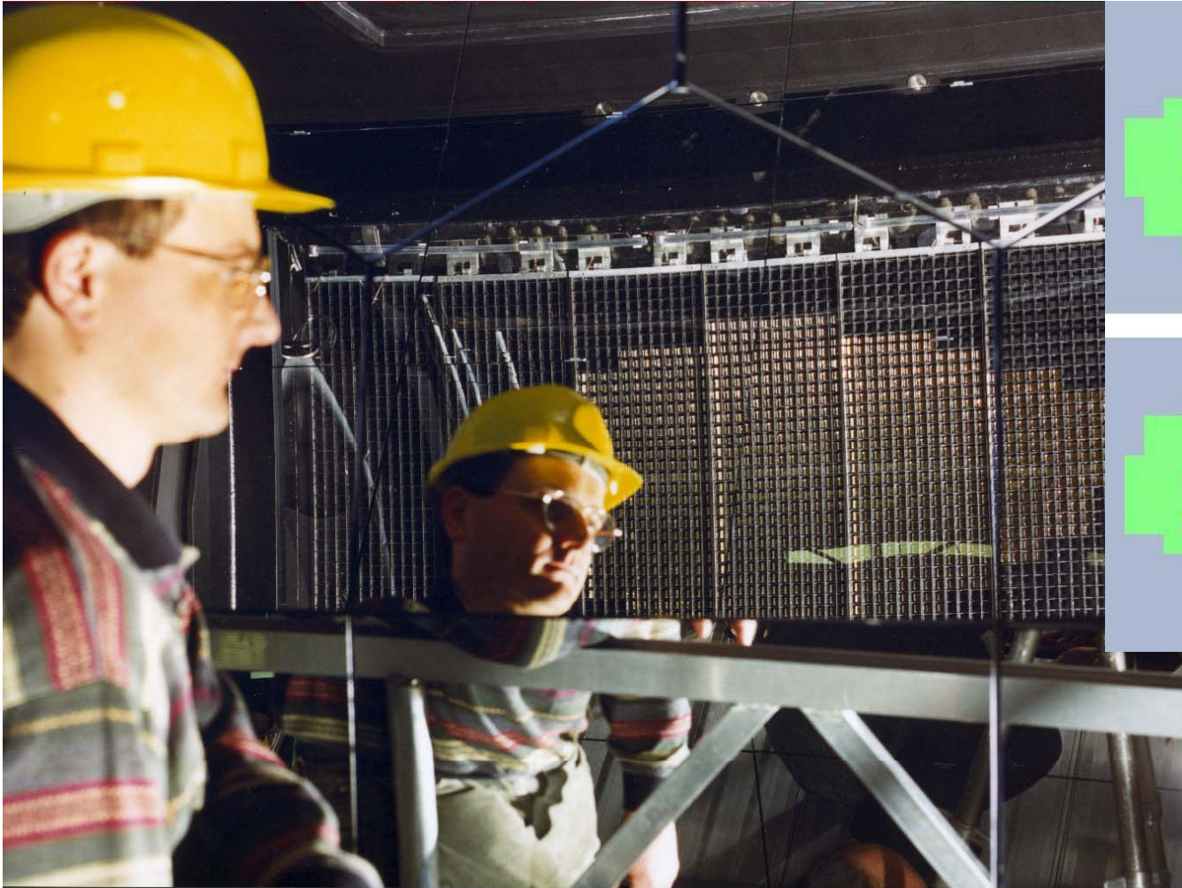
HERA-B RICH with 27 thousand channels (Hamamatsu R5900-00-M16)
