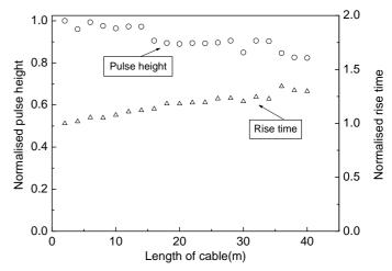
Fig. 6. Variation of the normalised pulse height and rise time with the cable length for a silicone coated P-120 grade bakelite RPC.
