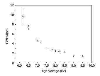
Fig. 8. The time resolution as a function of HV for a silicone coated P-120 grade bakelite RPC.
