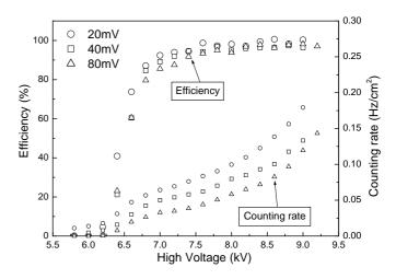
Fig. 2. The efficiency and the counting rate as a function of high voltage for a silicone coated RPC made of P-120 grade bakelite with discriminator threshold values of 20 mV, 40 mV and 80 mV. Used gas mixture is Argon (34%) + Isobutane (7%) + R-134a (59%).
