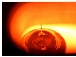
The difference between MCz-Si and Cz-Si is the magnetic field during the crystal growth. Magnetic field improves the controllability of the silicon melt thus improving the dopant/impurity concentration of resulting wafers.
