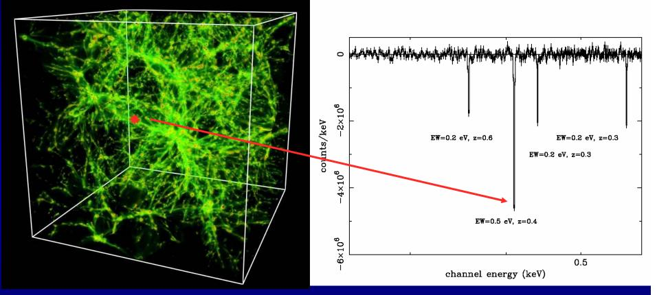
Simulations of WHIM absorption features from OVII as expected from filaments (at different z, with EW=0.2-0.5 eV from Hellsten et al 98) in the l.o.s. toward a GRB with Fluence=4 10<sup>-6</sup> as observed with ESTREMO/WFXRT (in 60 ksec). About 10% of GRB (10 events per year per 3sr).
