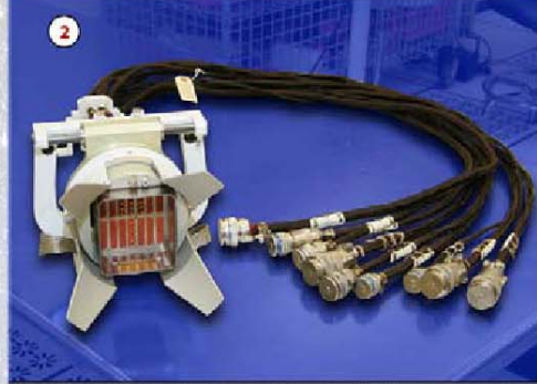
Remotely Operated Electrical Umbilical/ Payload Disconnect Assembly (ROEU/PDA)
