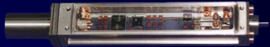
SQUID electronics in Niobium carrier
