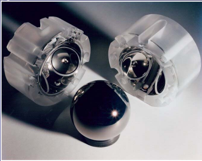
Gyroscope rotor and housing halves
