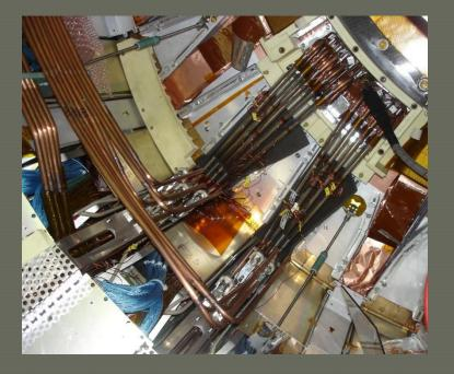
•Due to many failures and worry over the performance of the heaters, they were relocated to the cryostat face.
