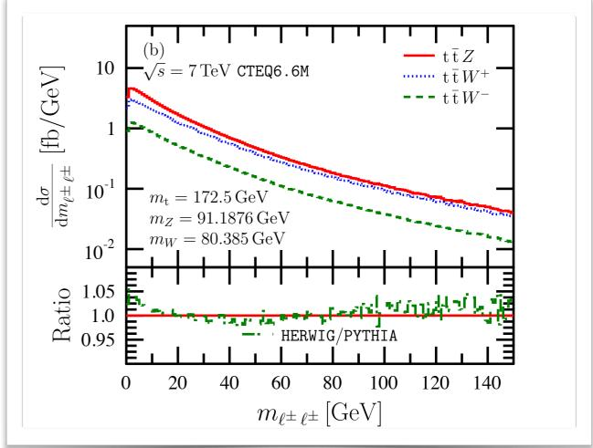
Invariant mass of all same flavour lepton-antilepton pairs and same-sign lepton and antilepton pairs at 7TeV LHC Selection of peak region used in trilepton analysis below
