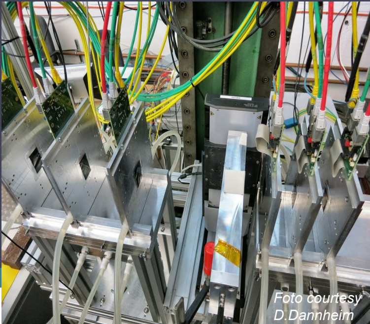
Top to bottom view on the EUDET telescope sensor fixtures with a DUT box mounted in between
