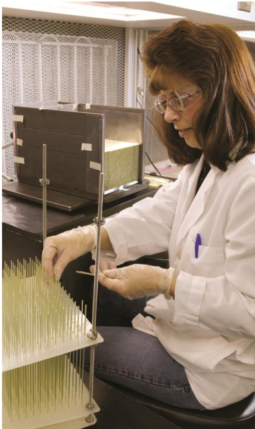
Multi fibers assembled in a shell
