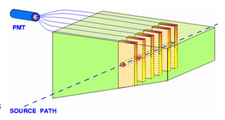
Cs calibration allows to equalise the channels response to a level of precision of 0.3%
