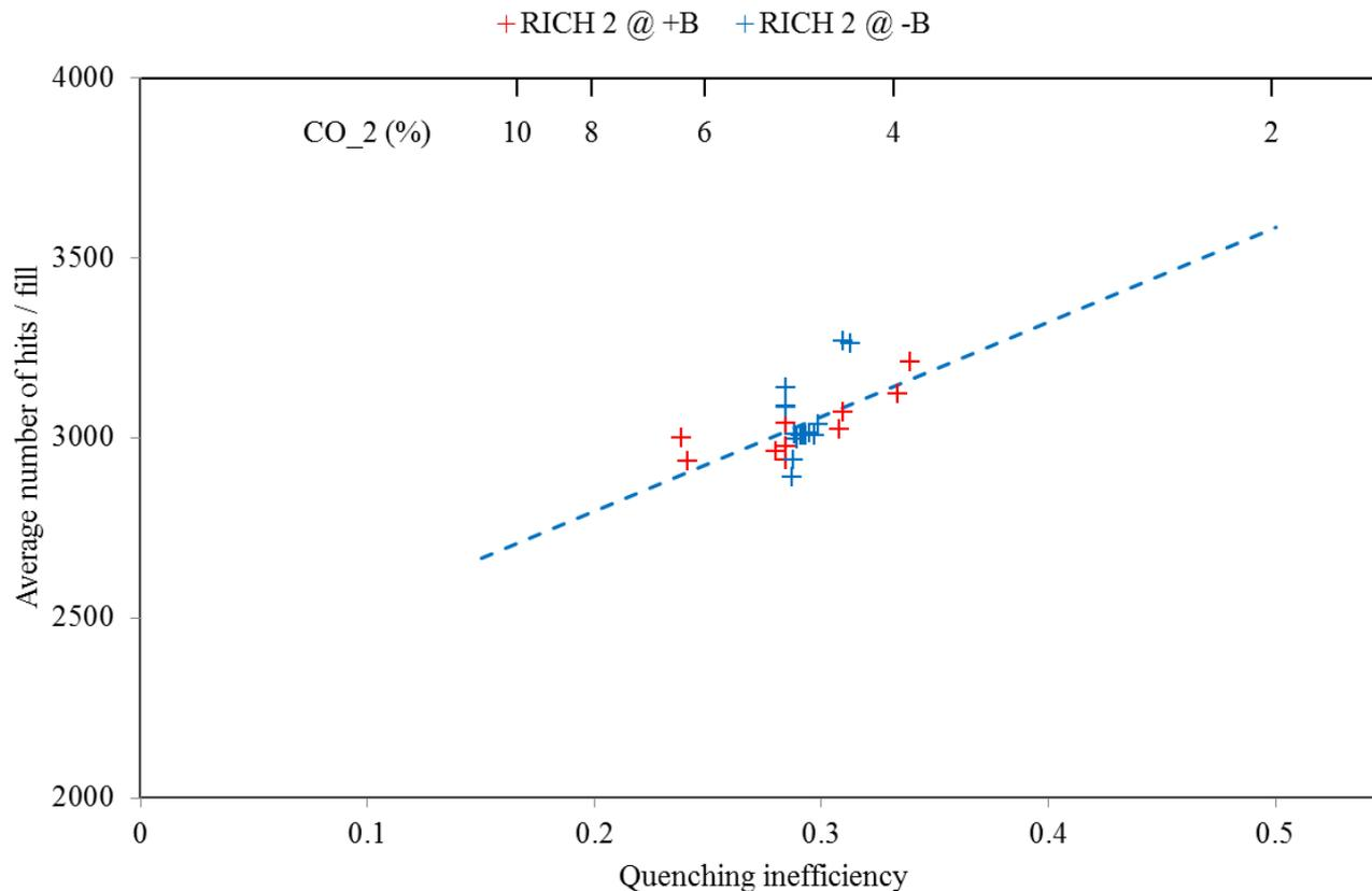
**Inefficiency is calculated from lab measurements**
