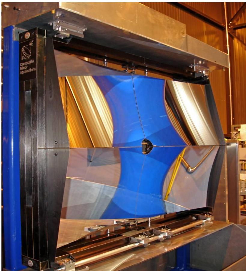
Carbon fibre mirrors for low material budget
