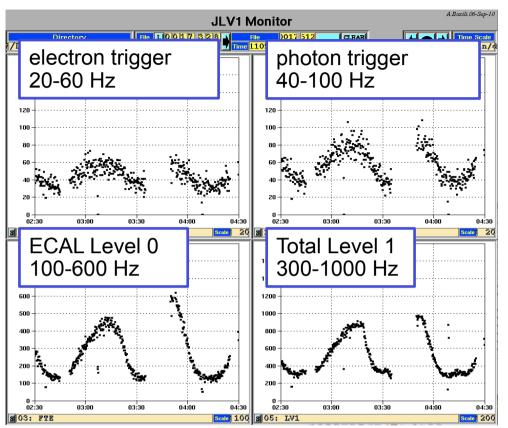
TRIGGER RATE – the photon trigger is ~10% of total Level 1 trigger, perfectly compatible with the design specification!
