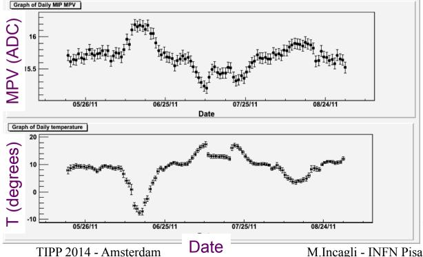
A dependence between MIP Most Probable Value (MPV = gain) and temperature was observed in flight data.
