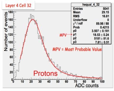
Cell equalization performed using proton and Helium Minimum Ionizing Particles (MIPs)
