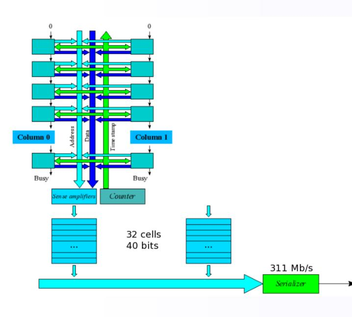
In Topix the pixels are organized in columns, with some electronics to store the events before the serialization. The present design foresees 110 column, each one arranging 116 cell. To save room on the layout, the same bus serves two adjacent columns transferring data towards the
