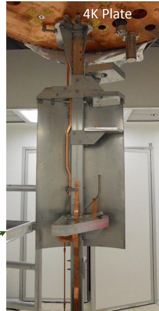
Stainless steel mockup for calibration system test NOT present in CUORE
