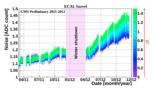
Energy equivalent noise (in MeV): noise in ADC is scaled by the laser corrections and IC
