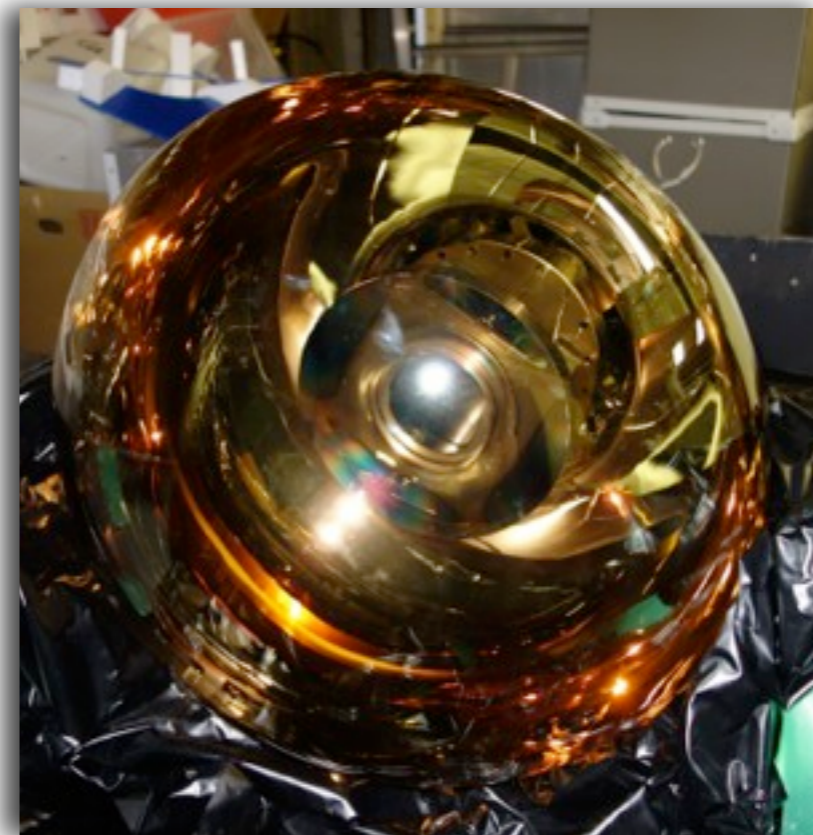
20" high-QE box&line PMT
