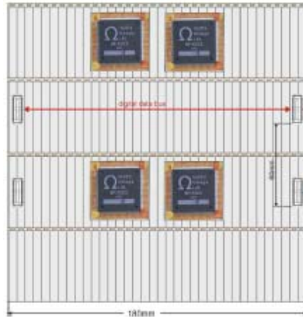
Placement of scintillator strips onto the EBU
