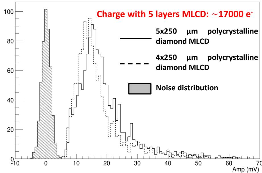
Adding a layer to the 4x250  $\mu\text{m}$  MLCD allows to increase the average induced charge of about 25%.
