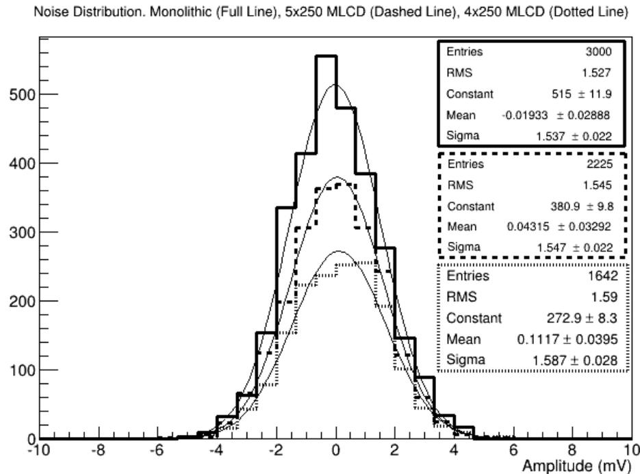
The 5 layers MLCD has exactly the same noise as the monolithic detector. The increase of detector capacitance did not affect the front end response.
