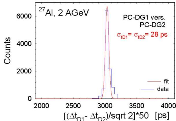
ToF measurement using Single Crystal Diamond Detectors on  $^{27}\text{Al}$  beam.
