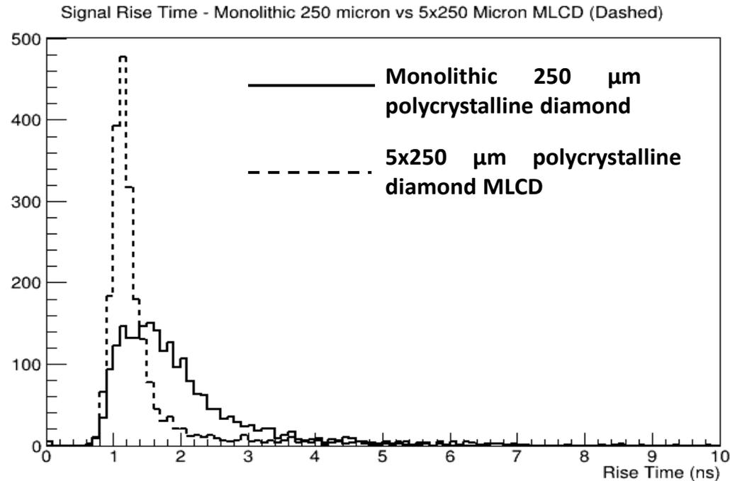
As expected the rise time depends only on the layer thickness. The multilayer structure does not deteriorate the rise time of the sensor. The signal rise time with the MLCD is even better than for the monolithic structure. The structure reduces the non-uniformities also for detector timing.
