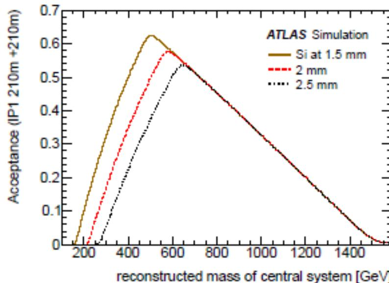
Acceptance of AFP as a function of the reconstructed mass of the central system at different distances from the beam.
