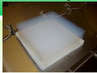
◆ index = 1.03 is suitable to get high efficiency for  $e^\pm$  (or  $\gamma$ ) while keeping detection of  $\pi^\pm$  and protons (or n) suppressed
