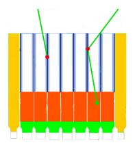
Active and passive collimators for point-source optimisation
