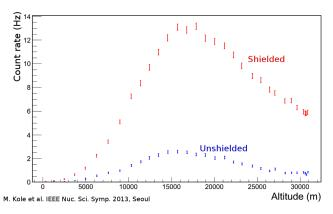
With 5 mm thick scintillator 300 second measurements suffice for a statistically significant measurement
