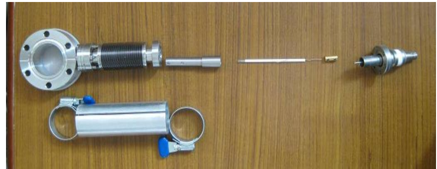
BNC feedthrough, copper connector, ceramic tube with bulb, stainless steel tube (ceramic tube holder), bellow and flange with port.
