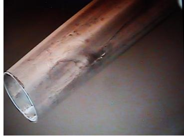
Not corrosion or pipe failure; just break of laser welds
