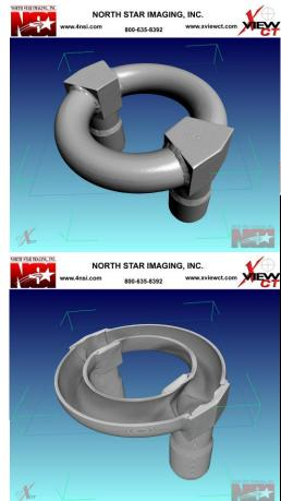
CT Scan to Qualify Downstream Turnaround Ring Weld Integrity (Difficult Geometry for Conventional X-ray Inspection)
