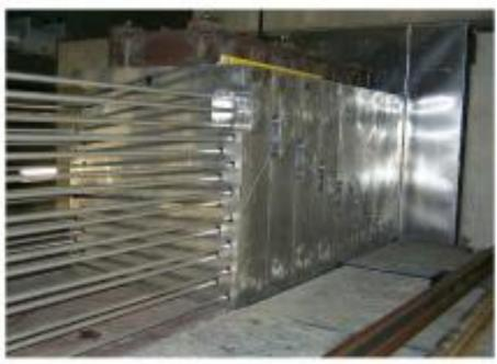
Thermocouples mounted in middle of core, at shower maximum, for monitoring.
