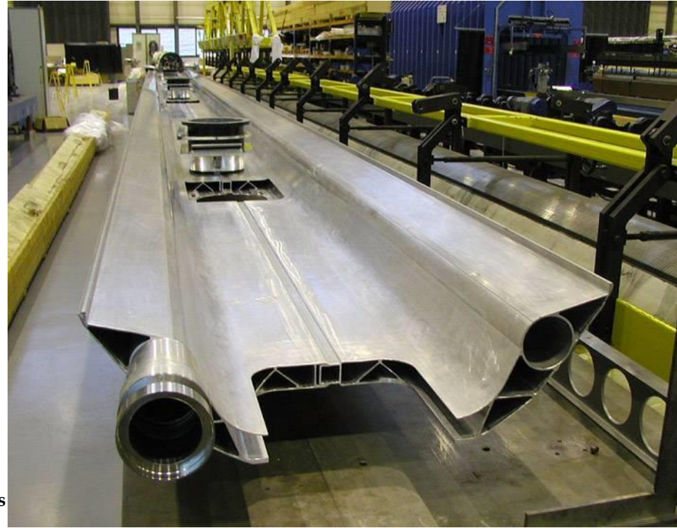
Aluminium alloy 6063 extrusions and 1100 top sheets
