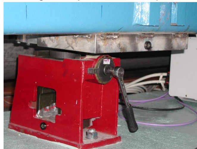
Alignment jacks under a dipole
