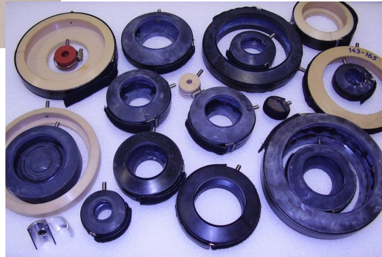
Clam-shells for pipe geometries for LHC
