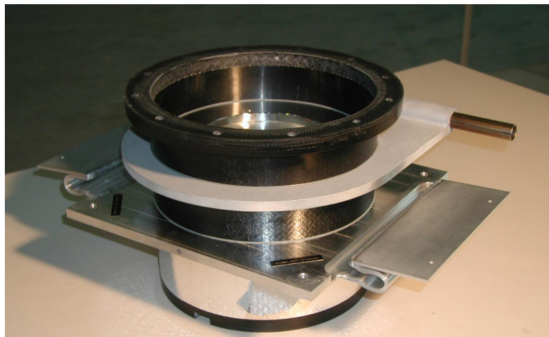
Low heat in-leaks support posts
