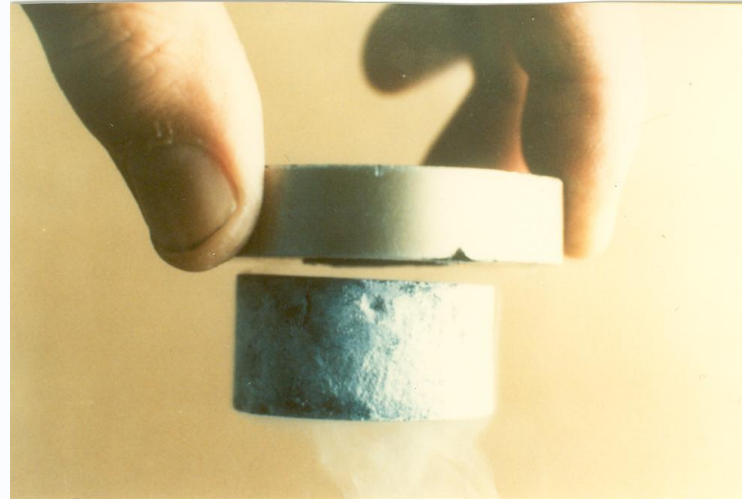
Levitating YBaCuO sample at 77K
