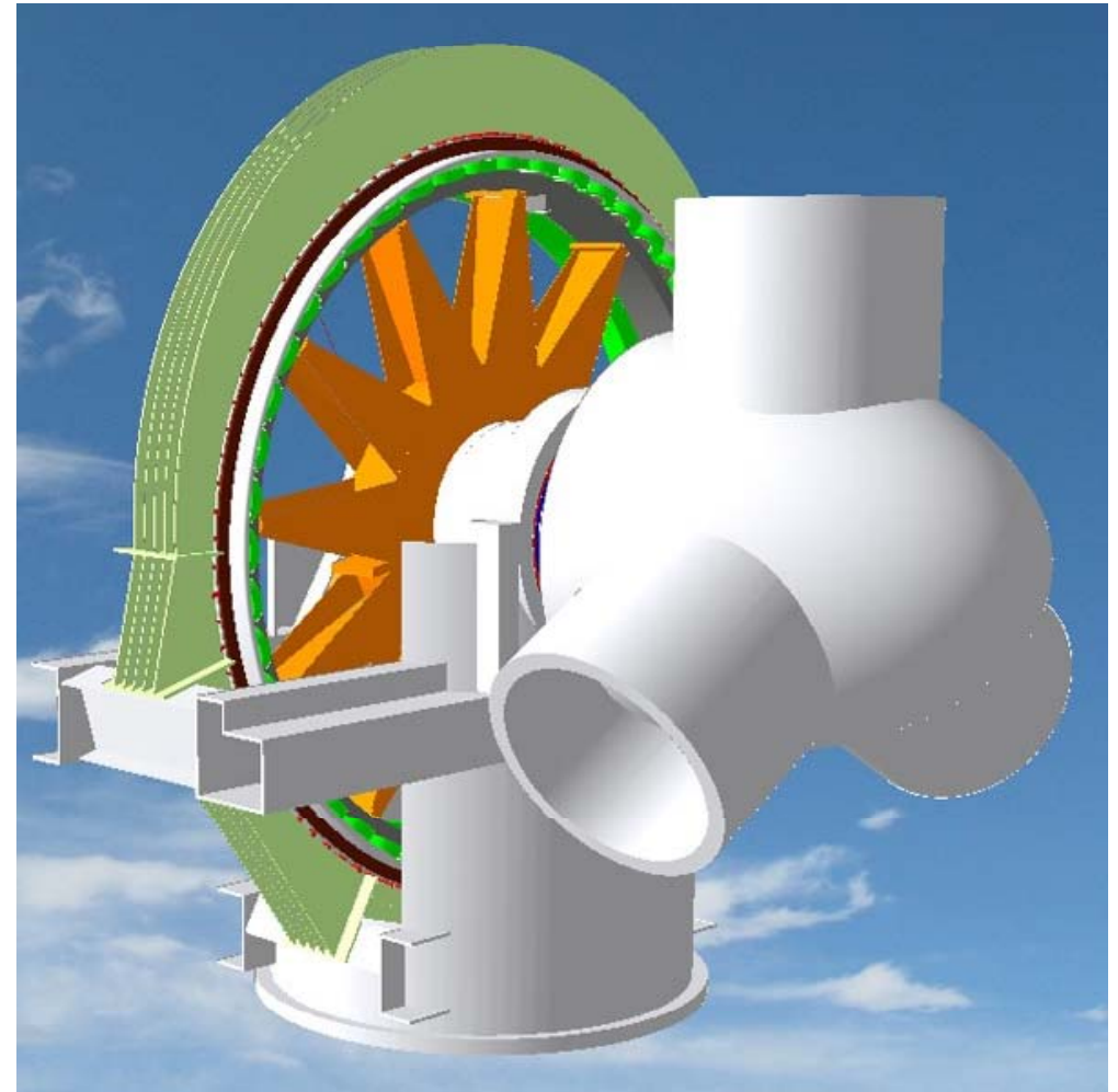
SC wind turbine according to Tecnia concept (PTC/ES2009/070639)
