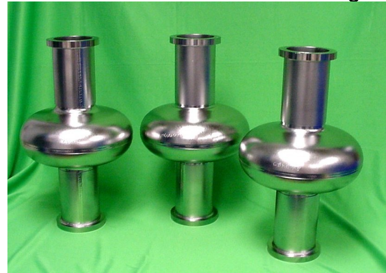
Single Crystal Cavities with three different crystal orientation
