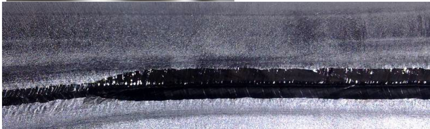
Repaired welding seam
