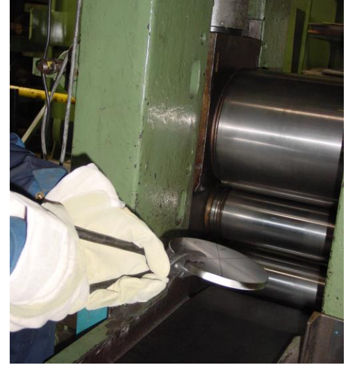
3. Increasing of diameter by special rolling with an intermediate annealing
