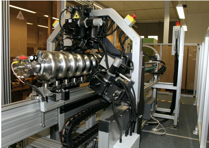
Optical control by high resolution camera
