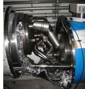
Damage at an LHC interconnect
