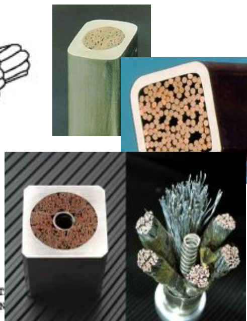
ROUND BUNDLE WITH 37 STRANDS ENCLOSED IN RECT CONDUIT - SHOWING TRANSPOSITION OF STRAN
