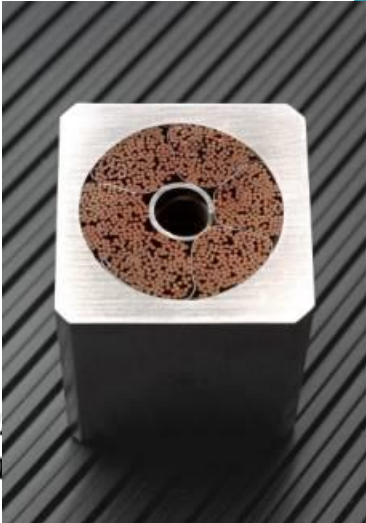
ROUND BUNDLE WITH 37 STRANDS ENCLOSED IN RECT CONDUIT - SHOWING TRANSPOSITION OF STRAN
