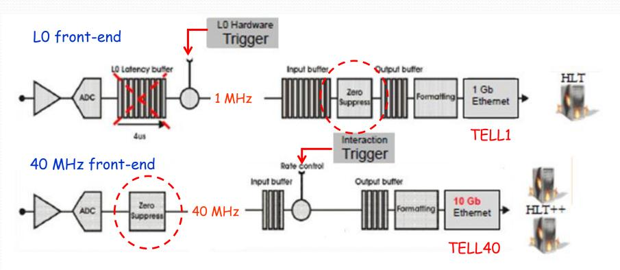
New front-end chip for the pixel/strip option New electronic acquisition board - TELL40
