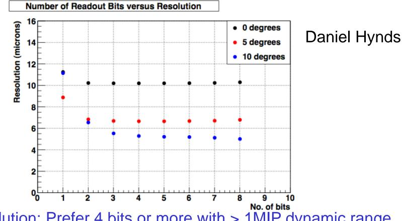
Resolution: Prefer 4 bits or more with > 1MIP dynamic range Additional bits for common mode & pedestal subtraction Baseline 6-bits
