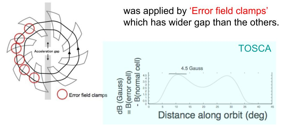
\* Effects of accelerations at two gaps work in counter-phase
