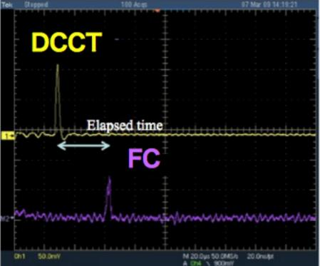
Elapsed time was measured at different radius
