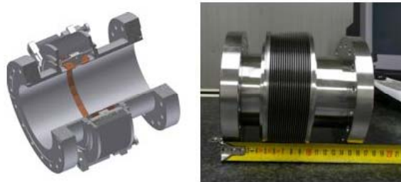
Figure 6: Copper-Beryllium strip shielded bellows, mechanical design (left) and real device (right).
