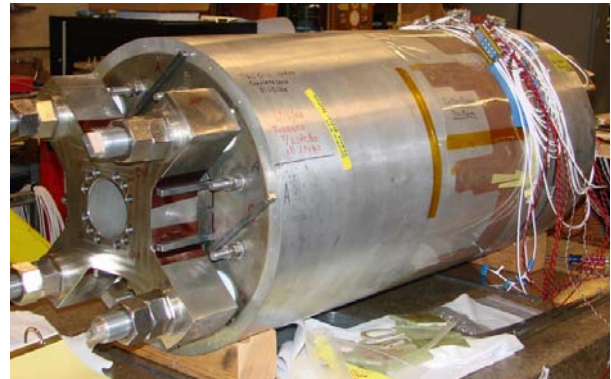
Fig. 4. Photograph of a TQS quadrupole cold mass
