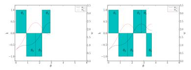
If we fix the gradient,  $L^*$  and  $\beta^*$  we can find the smaller possible beam size (beta peak) in the triplet or quadruplet.
