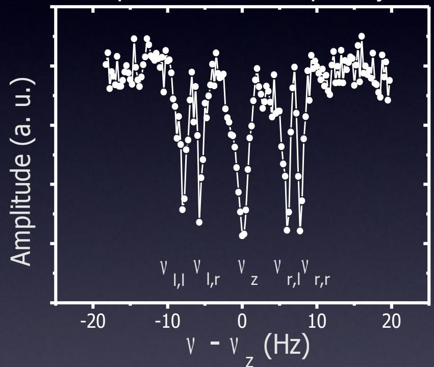
**FIRST DIRECT MEASUREMENT OF THE FREE CYCLOTRON FREQUENCY ( $\Delta\nu_c/\nu_c = 5*10^{-9}$ )**
