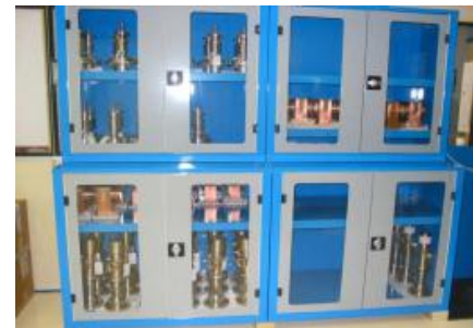
DESY coupler storage cabinet
