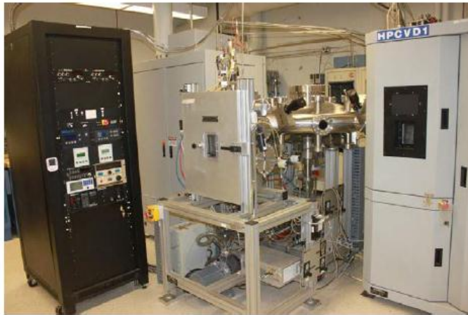
Integrated HPCVD system for cavity coating
