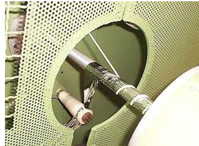
Automated winding of Superinsulation and Spacer
