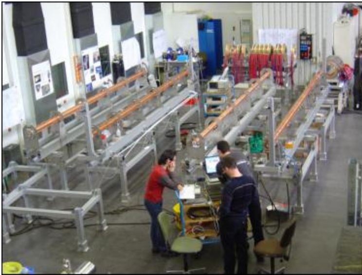
RF testing and assembly of linear accelerator systems
