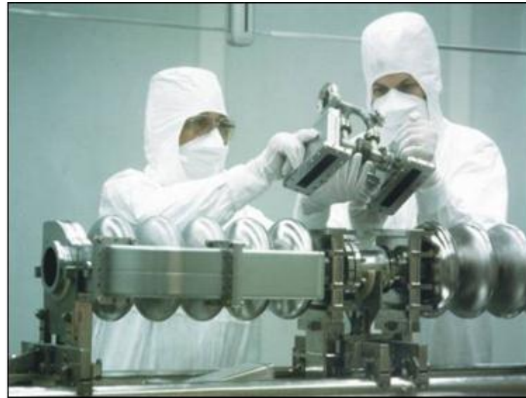
Assembly of superconducting rf structures in clean room condition (ISO 4)
