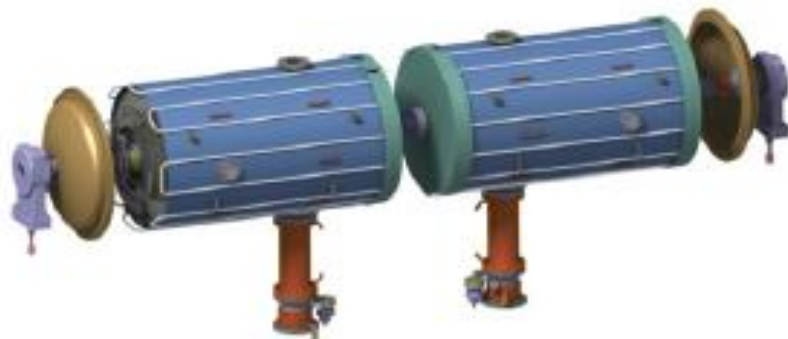
Cavity string and its cooled magnetic shielding
