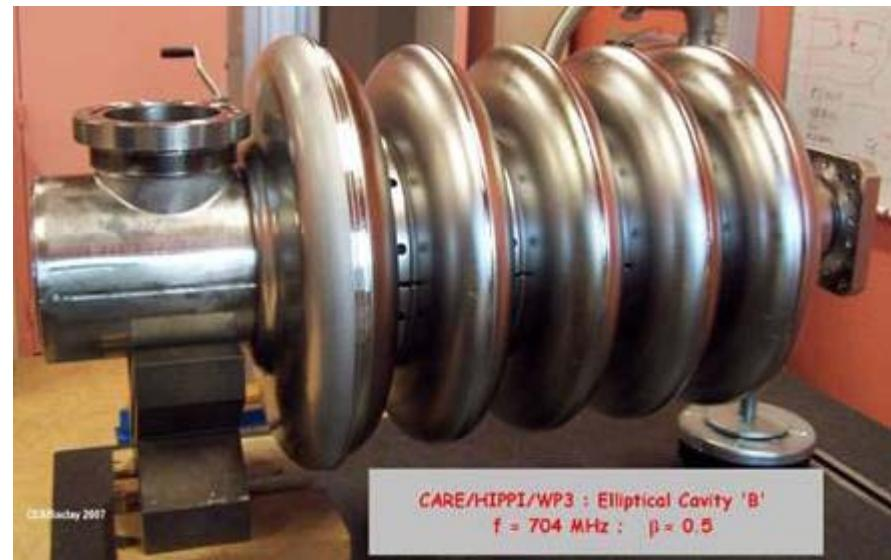
Cavity B , delivered in march 07 at Saclay, has been measured (frequency, bead pull) and it is now ready to be integrated in the CryHoLab environment.
