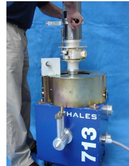
TH713 IOTs L band 16 kW cw
